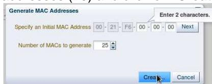
Note: Since the VirtualBox virtual machines network connections are “host only”, they cannot have access to external network, so we can use the same MAC addresses for the VNICs on the different laptops.
