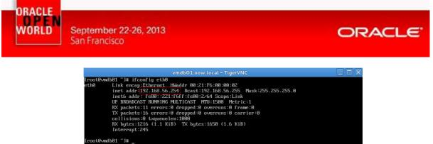
An alternative to see witch IP Address has been assigned to "vmdb01.oow.local" is:
